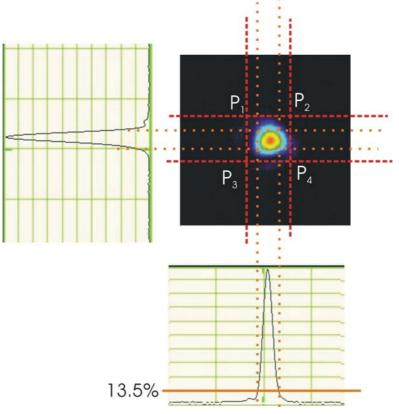
(i) from the horizontal and vertical profiles determine the Positions where the profiles cross the 13.5% level of the maximum intensity (x1,x2,y1,y2).
