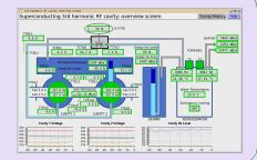
Qt-Designer extended by our plugins and caQtDM represent a good control system environment for developing and rendering control system data displays.
